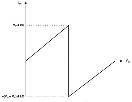
Figure 4. Typical I<sub>IN</sub> vs V<sub>IN</sub> Curve
