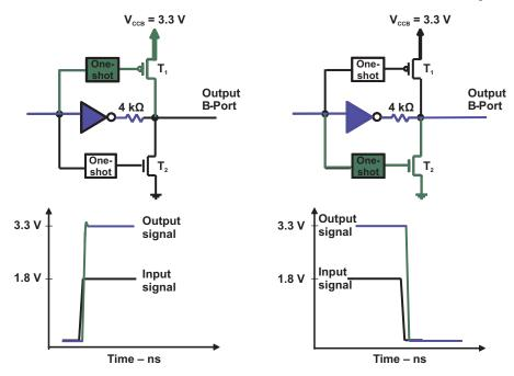
Figure 3. Active Output Rising/Falling Edge-Rate Acceleration Circuitry and DC Resistor Paths
