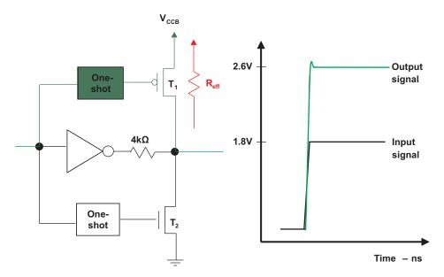
Figure 5. TXB Active Output Rising Edge-Rate Acceleration Illustration
