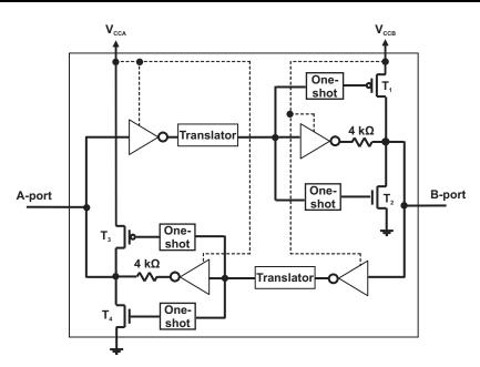
Figure 2. Basic TXB010x Architecture
