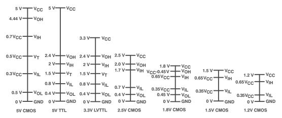
Figure 1. Digital Switching Levels
